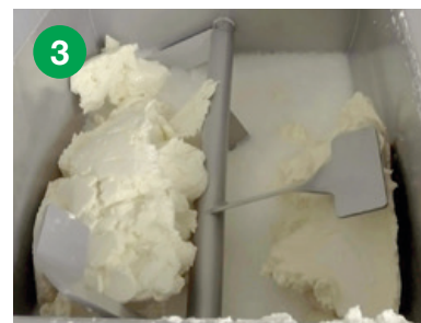
3 After 20 minutes, the buttermilk is secreted and discharged through the outlet valve.
